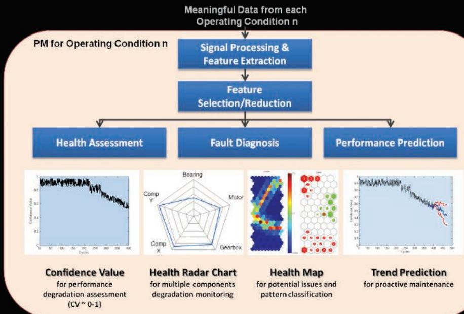
Wind-turbine behavioral tools may include routines for feature extraction, health assessment, and fault diagnostics, which have been studied and applied intensively by the IMS center for common rotary-machinery components, such as gearboxes and bearings. The results get displayed in visualization tools for degradation assessment and monitoring.
