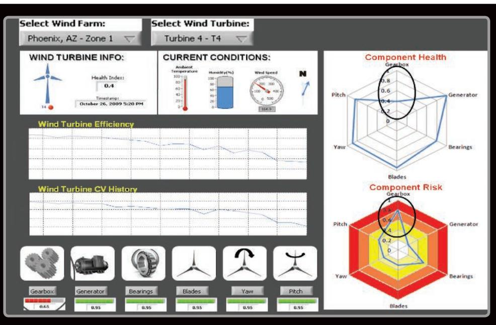
ponents (such as gearboxes, bearings, and rotor blades). Each axis on the chart shows the confidence value of a specific component.
