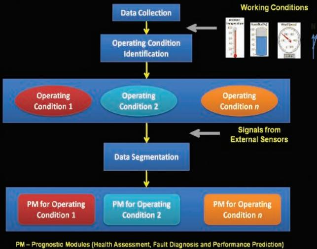
The modeling of a wind turbine for predictive maintenance starts with the collection of data, including those indicating real-time system-operating conditions, and using them to identify the system's regime of operation. With the operating regime identified, the data goes into the corresponding prognostics model that has either been established, or will have to be created for a newly learned operating regime.
